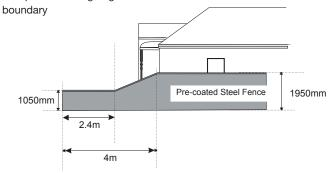
Boundary fencing between allotments (fence will taper to 1050mm commencing at the point located 4m from the boundary).
