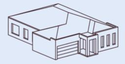
Flat roofs (pitch less than 10 deg) where the roof cladding is screened behind a parapet wall
